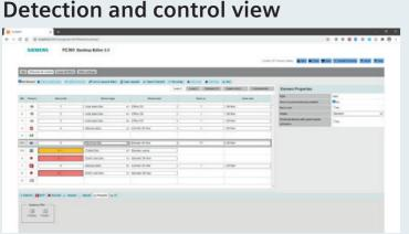
The FC360 configuration tool is simple to understand and use. The connected devices are listed in a table in their order of wiring, allowing the user to easily visualize the devices as installed. Outputs and sounders can be assigned into one of 32 control or evacuation zones and an appropriate description text (e.g. "door release") can be added for more clarity.
