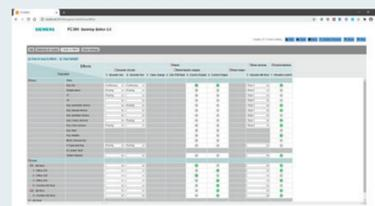
The FC360 configuration tool is simple to understand and use. The connected devices are listed in a table in their order of wiring, allowing the user to easily visualize the devices as installed. Outputs and sounders can be assigned into one of 32 control or evacuation zones and an appropriate description text (e.g. "door release") can be added for more clarity.
