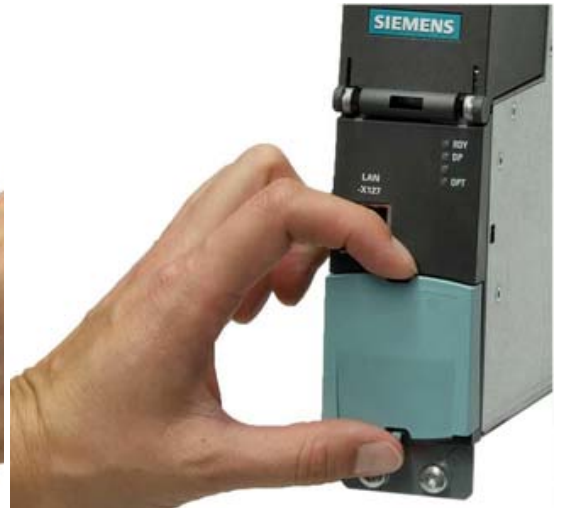
Remove the cover by pressing the latching cams together
