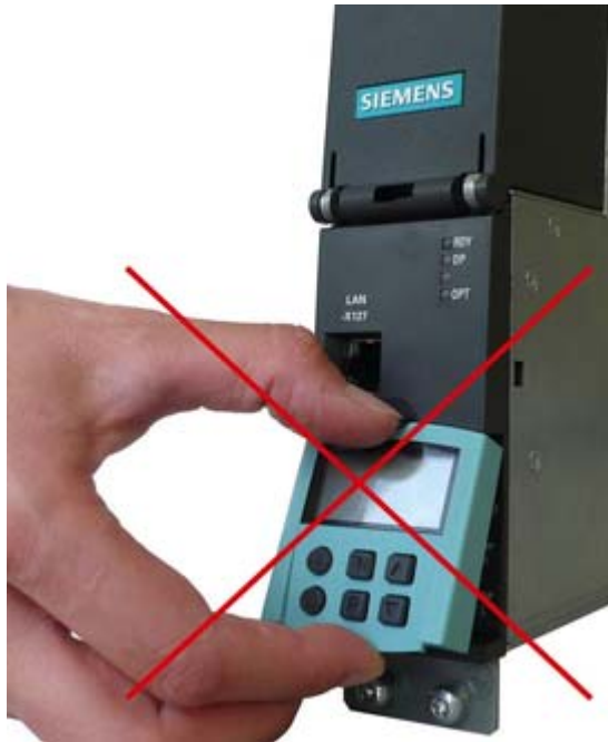
Figure 3-1 Incorrect mounting of the BOP20
