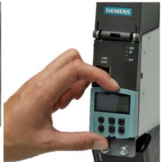
Carefully insert the BOP20 until you hear it latch into position
