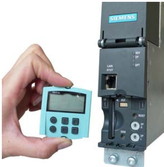
Insert the CompactFlash card before inserting the BOP20
