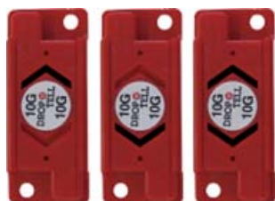
Figure 3-5 Shock indicator tripped
