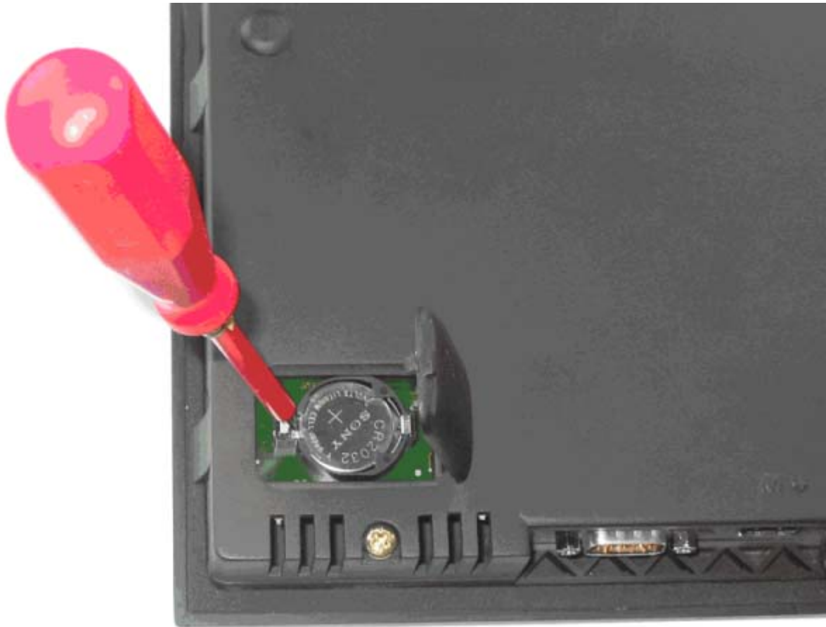
Figure 11-10 Replacing the backup battery for the cabinet operator panel
