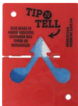
Figure 3-4 Tilt indicator tripped
