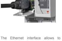
operate and configure the VMU-C, by means of LAN or direct connection to a PC, thanks to the integrated webinterface. In the case Ethernet cannot be accessed, the mini USB can be connected to a PC.
