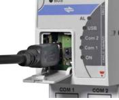
Since plant data are very important, VMU-C EM dedicates 4 GB of memory to secure data storage. VMU-C provides also a micro SD slot (up to 32 GB SDHC cards) and a hot-swap USB interface (for direct memory stick connection) on the top of the unit for: • plant configuration backup and
