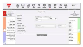
The database, including all the history of the plant, can be accessed to get a set of data in a defined time period. The data is then available in Excel compatible format for further analysis by the user.
