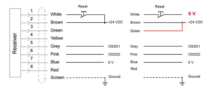
\*EDM (External Device Monitoring): monitoring of an actuator, a contactor for example, connected directly to the light guard.
