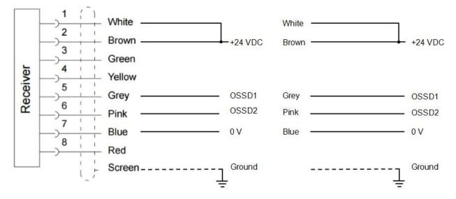
Reset button connected to the light curtain, no EDM\*
